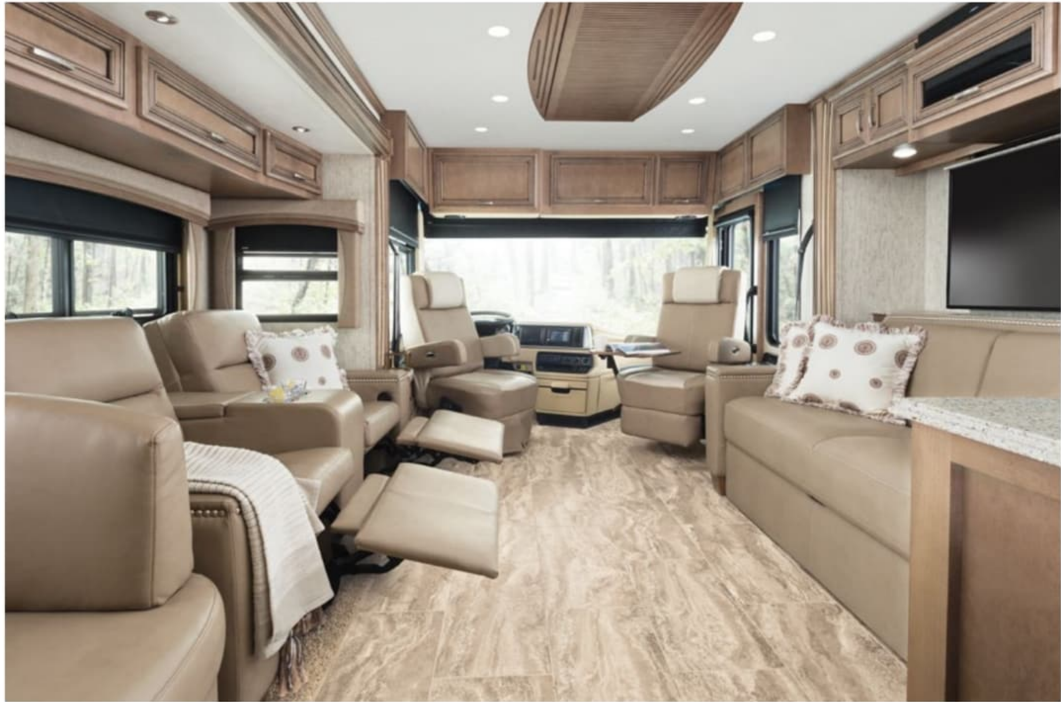
Grouted vinyl tile flooring
